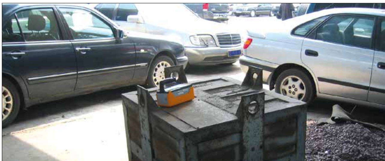
Disused teletherapy source stored without proper control / Credit: E. Reber (IAEA).
