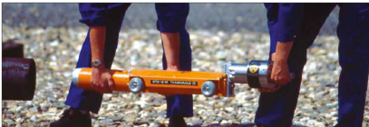
Pipeline crawler being loaded into an open pipeline / Credit: MDS Nordion.
